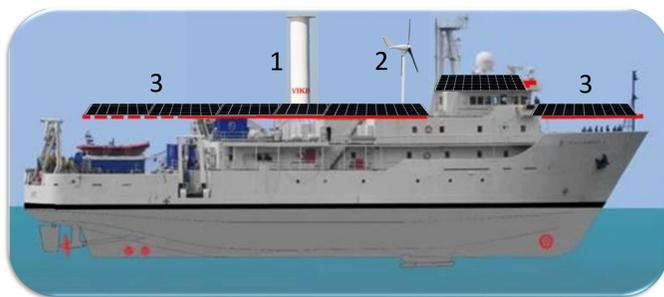
Figure 2. Ship external modifications (1 - Flettner rotor; 2 - Wind generators; 3 - PV panels).
